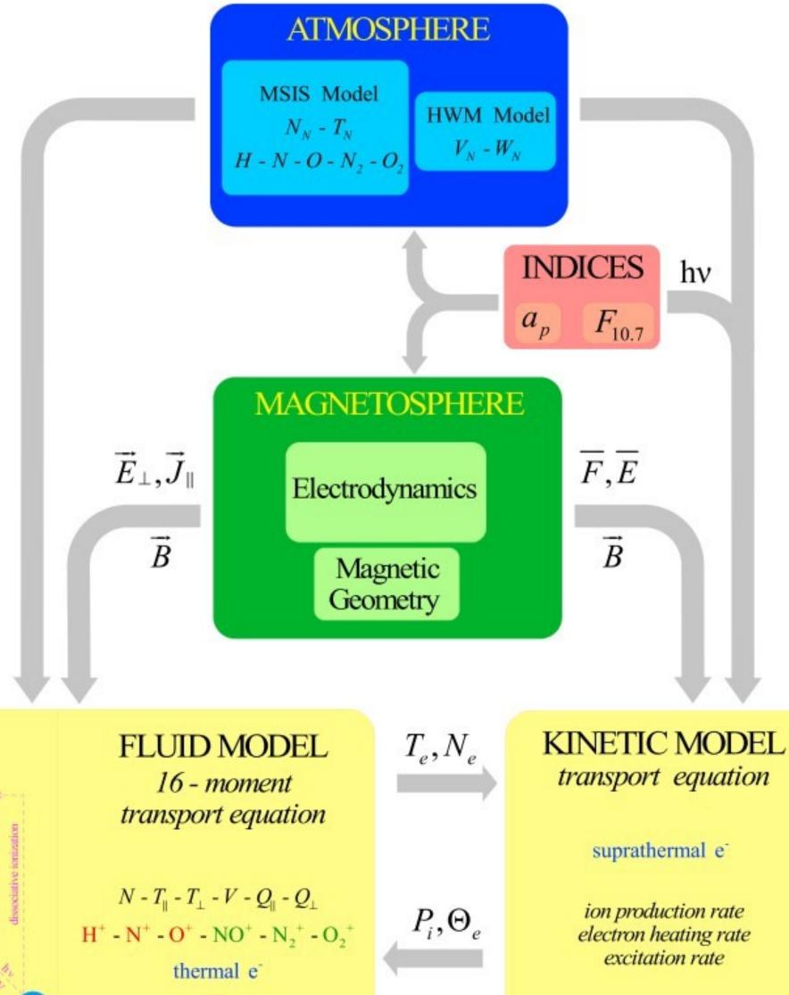
The fluid module computes the thermal electron density and temperature which is then passed to the kinetic part to return the ion production and thermal electron heating rates.
